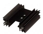
Smart Heatsinks, Inc. introduces the low cost, E-series, standard heat sinks for TO-220 and TO-218, devices. This simple heat sink can hold one TO device with adjustable height, and can be mounted simply by soldering onto PCB. The heat sink has two types of surface finishes, and can be used in either natural (free) or forced convection cooling applications. *Cross reference to AAVID P/N:* 531102B02500G Series.
